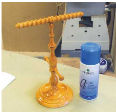
▲ Pic.35 For a glossy finish Les omits sanding sealer on this dense timber, and applies lacquer followed by burnishing cream when the lacquer is dry
